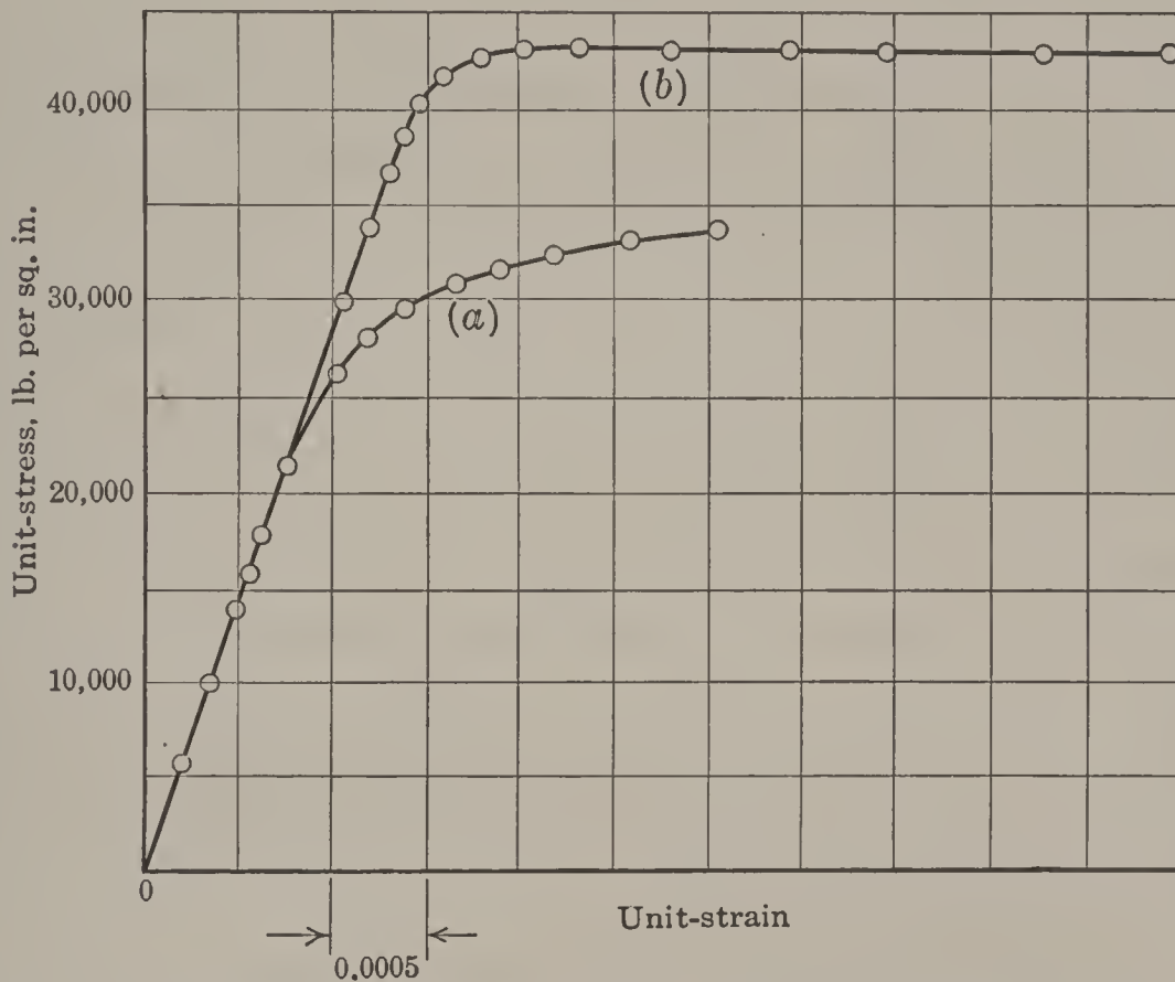
FIG. 253.—Stress-strain diagrams of steel casting and rolled steel showing the effect of the hot-working. (a) Specimen from steel casting that cooled slowly after being poured. (b) Specimen of same chemical composition as (a), steel rolled while cooling.
